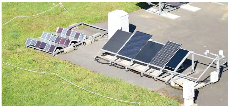
Figure 24. Photovoltaic test bench installed on the Sirta climate observatory operated by IPSL allowing simultaneous measurement of photovoltaic production and the weather variables affecting it
